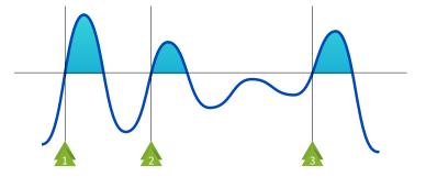
Stop missing events due to an uncalibrated front-end. Felix offers the possibility to adapt to every need through a programmable variable threshold comparator. In this way, you can precisely control the voltage level which triggers the time measurement.
